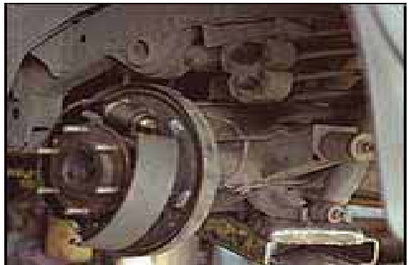
Figure 4: Brakes containing asbestos rope products
